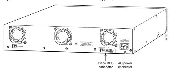
Figure 12 RPS 8-Pin Connector Location on a Cisco Router or Concentrator (Typical)
